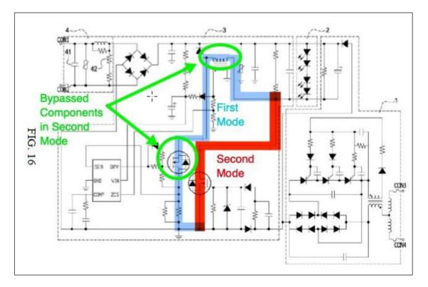
Petitioner provides an annotated version of Figure 16, reproduced above, which circuits are bypassed (in green) in the alleged First Mode of operating Duan (in blue) as opposed to the Second Mode of operating (in red). *Id.*
