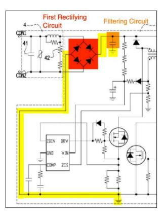
Petitioner's annotated portion of Figure 16, reproduced above, illustrates the location of the alleged filtering capacitor (orange) and the circuit path (yellow) to the alleged first rectifying circuit (red).
